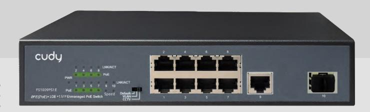
8-Port 10/100M(PSE)+ 1 Gigabit Combo Port unmanaged PoE Switch
