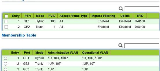
3. Configure the Switch A's interfaces by default, namely all interfaces access VLAN1 in an Untagged way. Connect the MAC addresses of PC1, 2 and 3 with VLAN10. Click the "VLAN > MAC VLAN > MAC Group" in the navigation bar, enter the MAC addresses of PC1 (0022-0022-0022), PC2 (0033-0033-0033) and PC3 (0044-0044-0044), with the mask of 48-bit exact match as follows:
