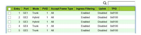
3. Add the Untagged GE2 and GE3 to VLAN10 and VLAN20 respectively. Click the "VLAN > VLAN > VLAN Configuration", drop down the list to choose VLAN10 and the Untagged GE2 port. Following the same steps, add the untagged GE3 to VLAN20 as follows:
