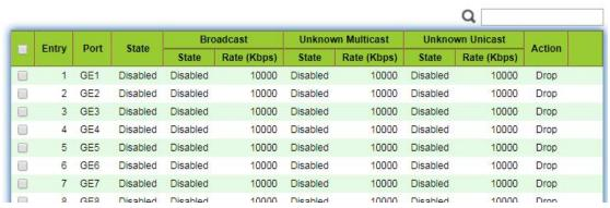
3. Configure info such as storm switch and rate, "Apply" and finish as follows:
