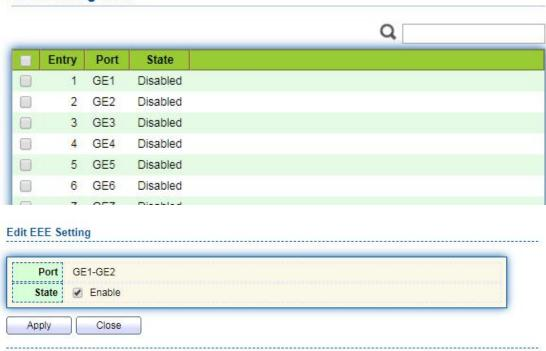
2. Set the port enable tag and "Apply" to complete the configuration as follows:
