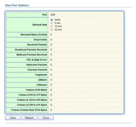
3. Select the specified refresh frequency to operate automatically.
