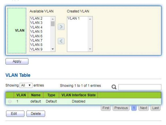
2. The VLAN created will be displayed in the VLAN Table. Users can "Edit" the VLAN as follows:
