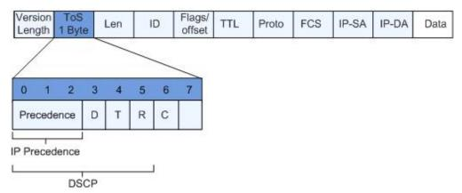
0 to 2 bits are Precedence fields representing the 8 priorities of message transmission ranging from 7 to 0 from high to low, with either Level 7 or 6 as the highest priority that is generally reserved for routing or updating network control communication. User-level applications only have access to Level 0 to 5.
