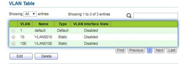
2. Configure Switch's GE1 in Hybrid mode with PVID of 100 to serve as an Untagged member of VLAN10. Configure GE2 in Trunk mode to serve as a Tagged member of VLAN10.
