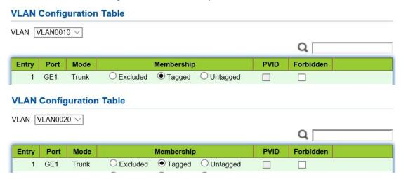
6. Related protocol and VLAN. VLAN IDs are assigned according to the protocol (family) type and encapsulation format of the messages received by interfaces. Click the "VLAN > Protocol VLAN > Protocol Group" in the navigation bar to add 2 rules for protocol groups:
