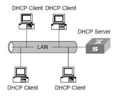
Figure 1-1. In a typical application of DHCP
