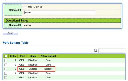
4. Configure on the port GE3 so that the circuit ID can be set by Option 82. Click the "Security > DHCP Snooping > Option82 Circuit ID" to configure the port. "Apply" and finish as follows:
