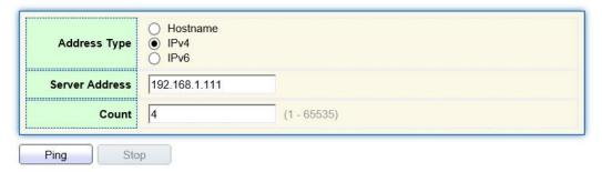
2. Click the "Ping" to accept the packet-transmitting test from system to verify address validity, and output the result as follows:
