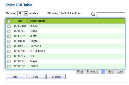
For example, configure the Voice VLAN in manual mode so that the ports accessing IP telephony can ingress/egress the Voice VLAN and transmit voice flow within it. Create VLAN2 to operate Voice VLAN securely, which allows only Voice Data to flow through. IP telephony transmits Untagged voice flow to GE1, the ingress Trunk port. Users must customize an OUI (0011-2231-05e1) and configure the Voice VLAN networking diagram in automatic mode.
