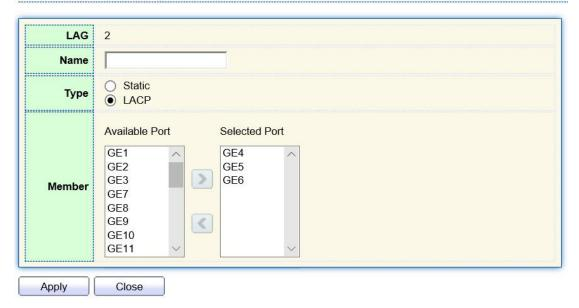
2. Click the "Port >Link Aggregation > LACP" in the navigation bar to configure the LACP attributes such as system priority, port priority and timeout method as follows:
