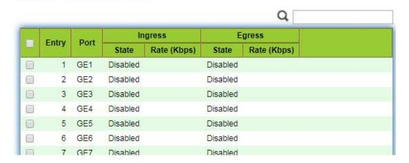
2. Select the port (s) for rate limiting, "Edit" it at the bottom to switch the function and specify the rate. "Apply" and finish as follows:
