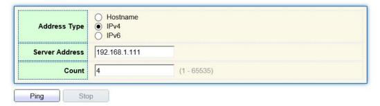
2. Click the "Ping" to accept the packet-transmitting test from system to verify address validity, and output the result as follows:
